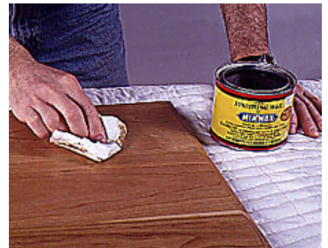
5- Once the last oil coat is dry, apply a light coat of paste wax to your project. Be sure to cover all the surfaces.
