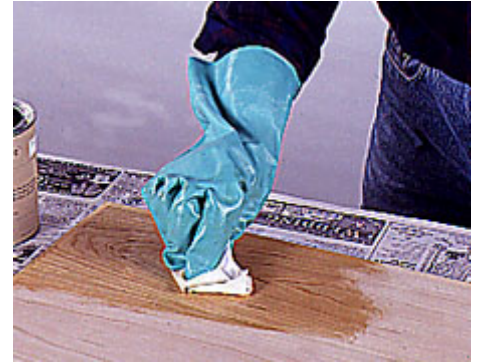
3- Apply an oil finish with a lint-free rag. Rub the oil into the wood and let it dry for 1 hour. Then wipe off the excess.
